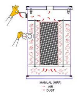
The Manual Reverse Purge (MRP) System allows for the cleaning of caked-on powder off of the filter thus maximizing performance. The filter cleaning is achieved by having the air intake reversed through the filter thus purging the clogged filter.
